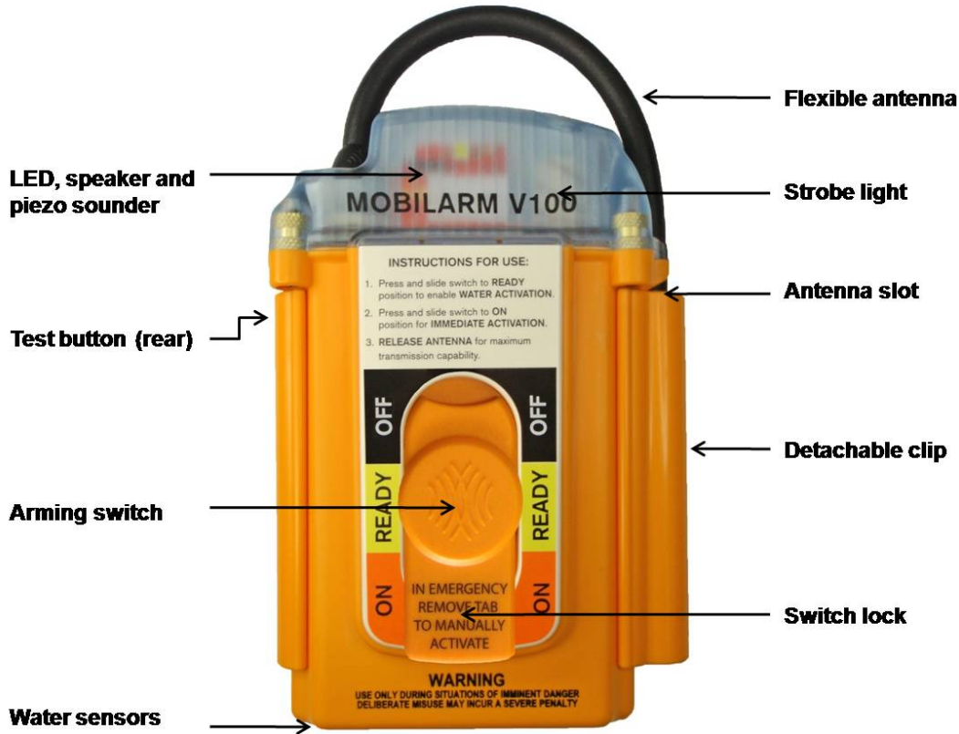
Figure 4: Crewsafe V100 features and controls
