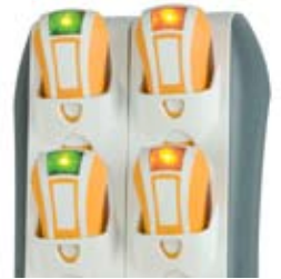
Tag LED indicates charging (orange) or fully charged (green)
