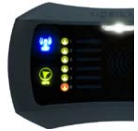
Alarm notification via strobe, audio alert and LED display
