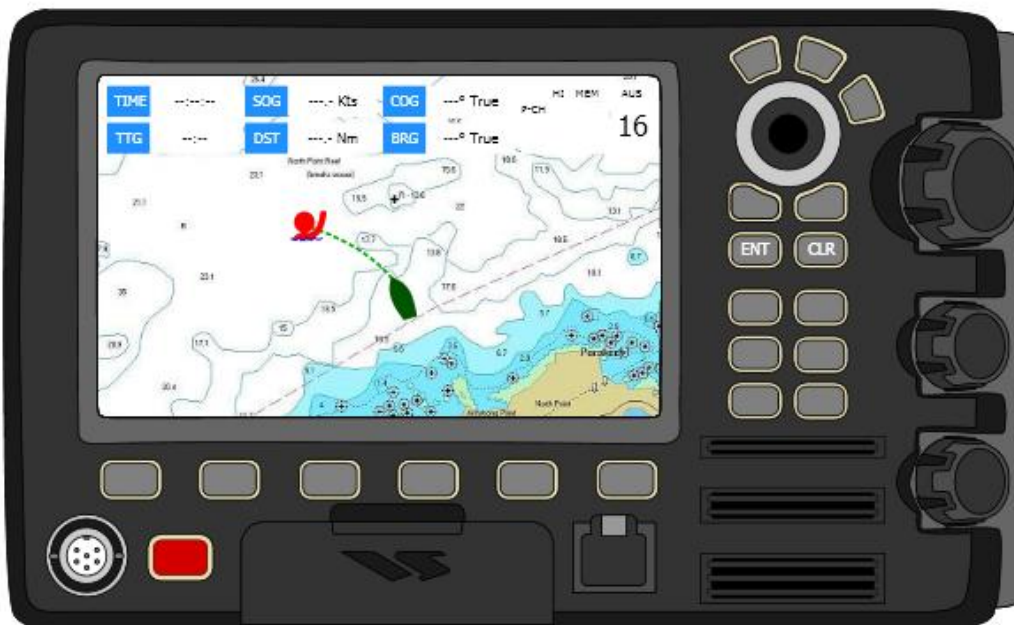
Chart plotter display screen, showing distance and bearing information
